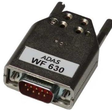
The WF630 module is a terminating load for dual redundant Digibus in compliance with the standard GAM-T-101:
