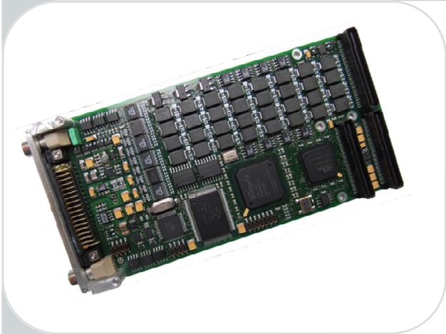
The PMC-AR429 interface board supports a full implementation of the communication bus ARINC 429.
