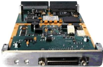
The front panel is delivered with each board. It can be mounted when the board is installed in an air cooled system with front connections. It supports a 50 pin female Honda HDR connector. Besides DIGIBUS and IRIG B the connector supports configurable inputs and output: two TTL signals and one RS422 signal in each direction. These signals can be affected by software to events such as message detection, cycle top or user's signal.
